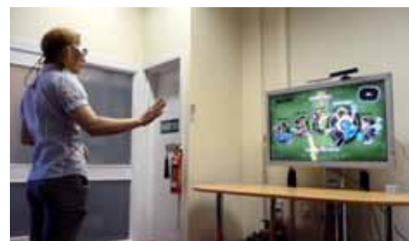
Image of the test set-up, with Xbox 360, Kinect and a player wearing the Tobii Glasses.
