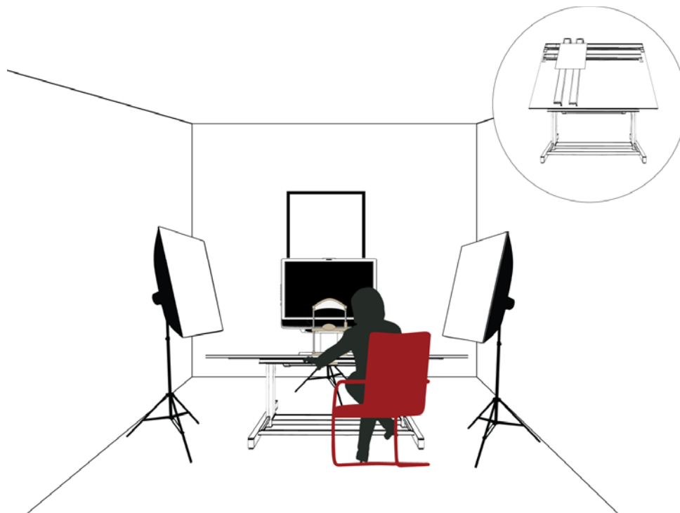
Figure 1, Test setup in the lab. The measurement setup is based on an XYZ-table (illustration in the upper, right corner in the image), and allows the eye tracker to be transferred to the specific positions in the head position tests. The participant is positioned in front of the eye tracker, using a chinrest in order to fixate the eyes' location. The lamps with soft boxes are positioned around the table to create an even light-spread in the room (for more details on the lab and test setup please contact Tobii Support to receive a copy of the Test Specification document.)
